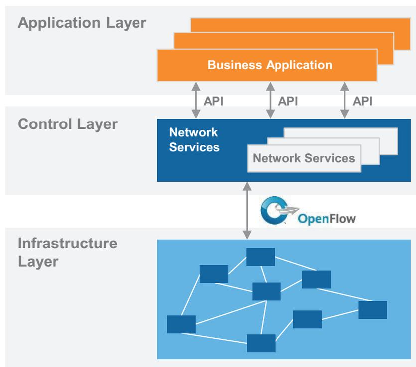
Figure: The SDN architecture
