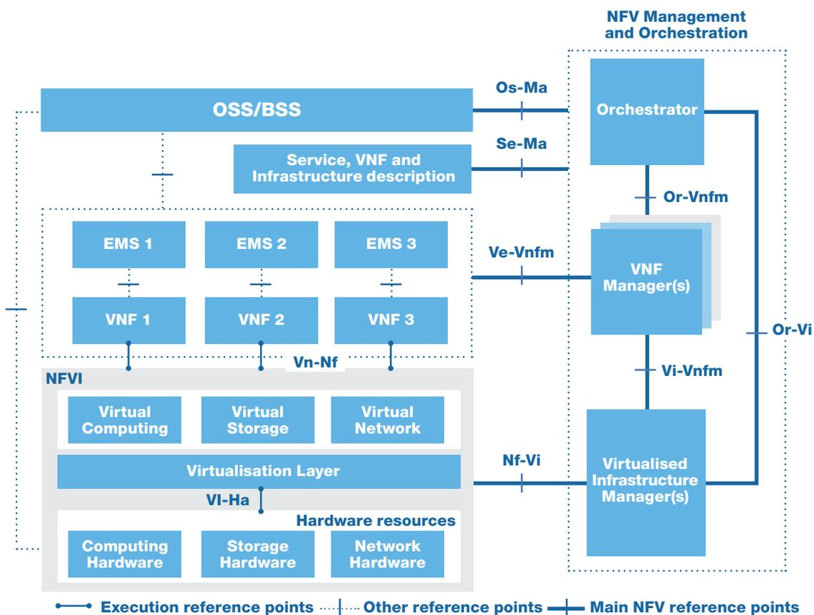
Figure: The ETSI NFV architecture
