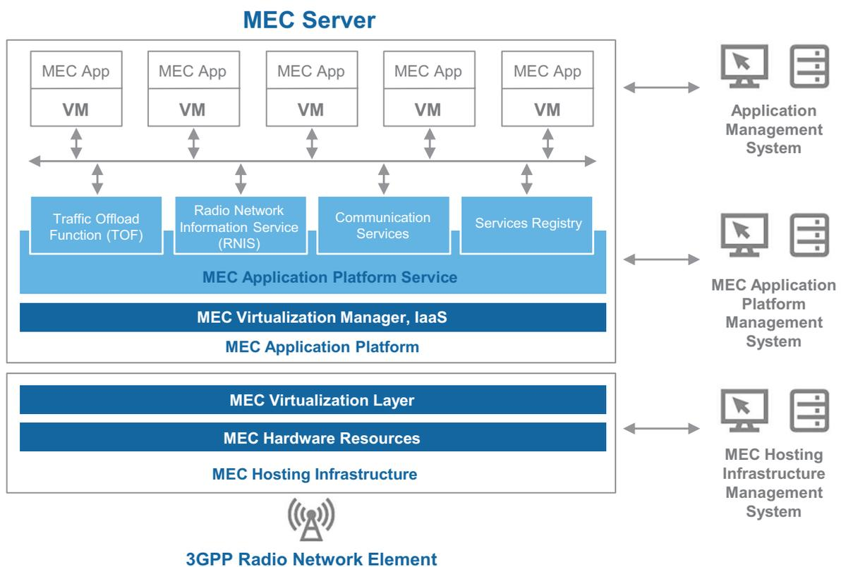
Figure: The MEC architecture
